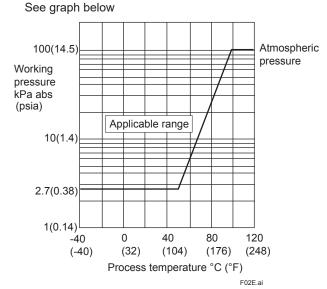
Figure 1. Working Pressure and Process Temperature
